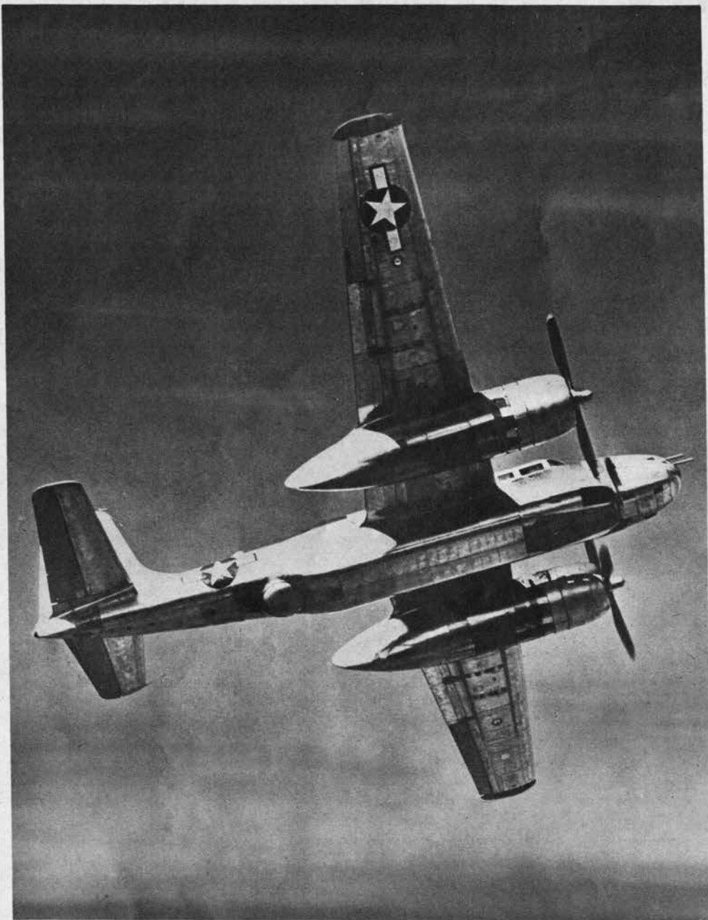
Square edges of wings and control surfaces give the A-26 a distinct personality from the A-20 Havoc. The remotely controlled turret in the belly breaks bottom line of fuselage.
